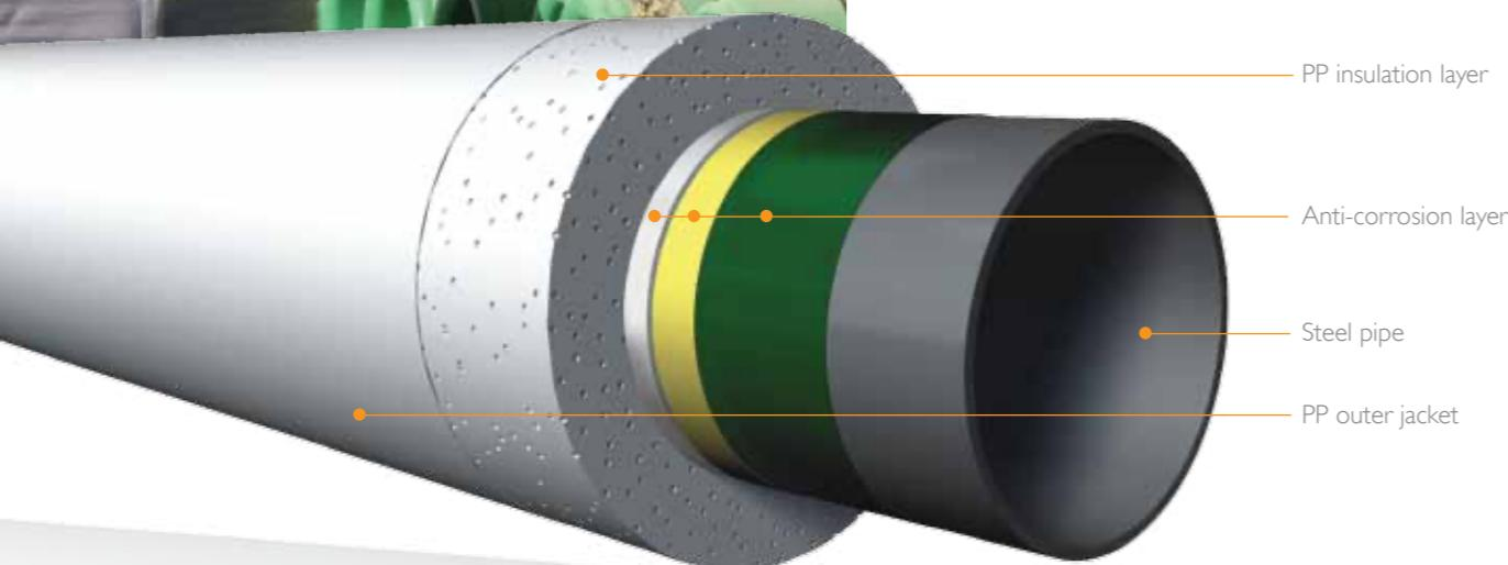
of each project. Then, and without this setting a limit, this combination of materials enables to reach maximum operation temperatures up to 140 °C in sea depths deeper than 3,000 meters, also adding anti-corrosive protection and mechanical resistance.
